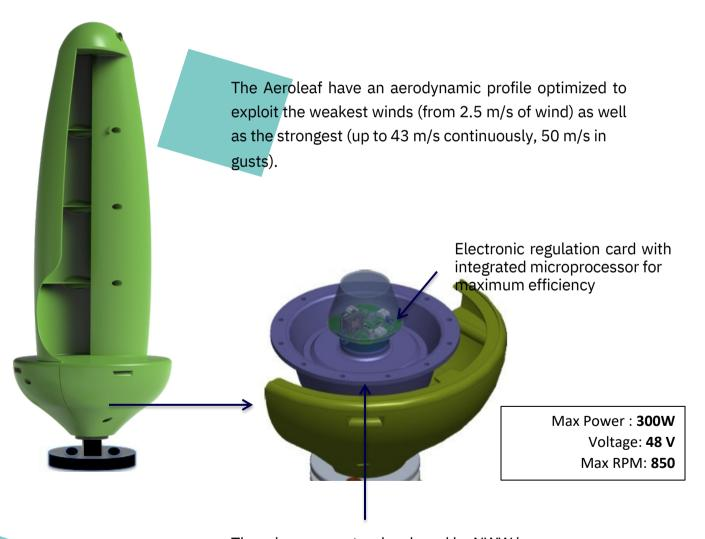
The micro generator developed by NWW is encapsulated in a casting to make it insensitive to the most aggressive environments: rain, sand, snow, pollution, salty air.
